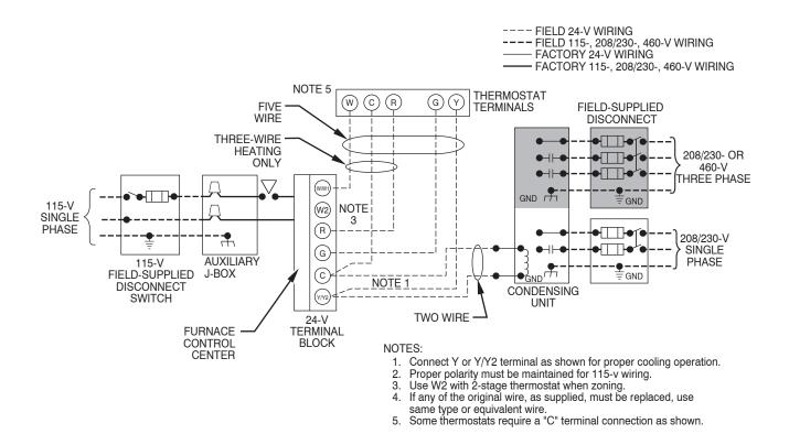
Fig. 27—Heating and Cooling Application Wiring Diagram
